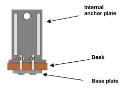
**4.** Place the external cover over the internal anchor plate.
